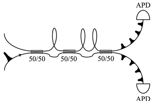
Fig. 1. Schematic setup of the detector. 50/50, symmetric fiber couplers.
