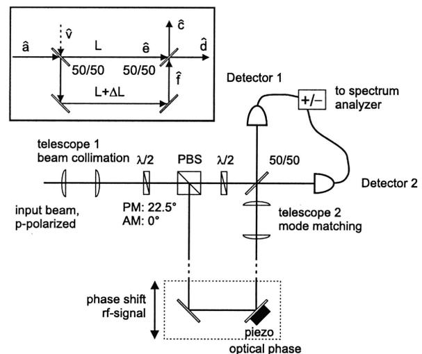
Fig. 1. Experimental setup of the phase-measuring interferometer. The orientation of the first  $\lambda/2$ -plate determines the type of measurement: amplitude measurement (AM) or phase measurement (PM). PBS, polarizing beam splitter; 50/50, beam splitter.
