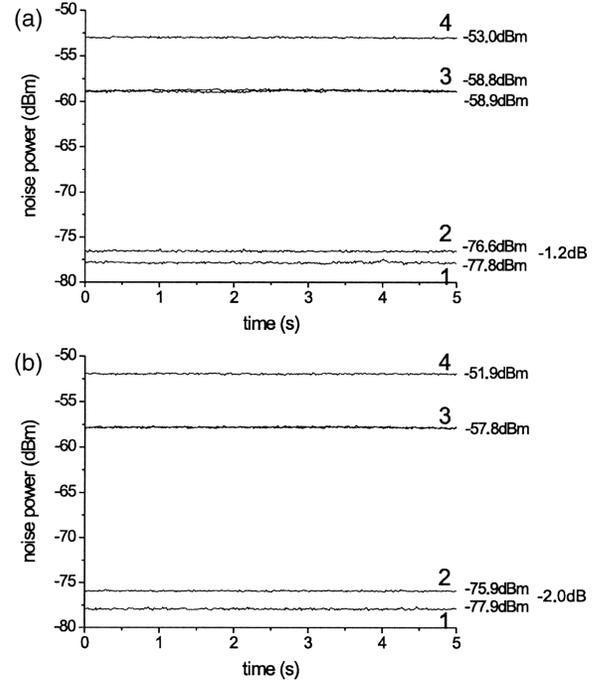
Fig. 2. Correlations of the (a) phase quadrature and (b) amplitude quadrature. In each graph the noise level (traces 1) of the correlation signal is shown together with the corresponding shot-noise level (traces 2), the noise level of the individual beams (traces 3), and the signal with the anticorrelations (traces 4). The traces were corrected by subtracting the electronic noise, which was at  $-84.7$  dBm.
