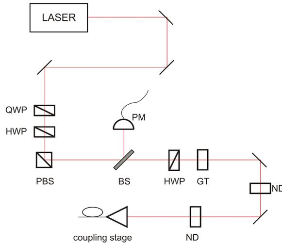
**Figure 1.** Scheme of the optical setup we used for characterizing the APDs in cw and pulsed operation: QWP, quarter-wave plate; HWP, half-wave plate; PBS, polarizing beam splitter; BS, beam splitter; PM, power meter; GT, Glan–Thompson polarizer; ND, neutral density filter.
