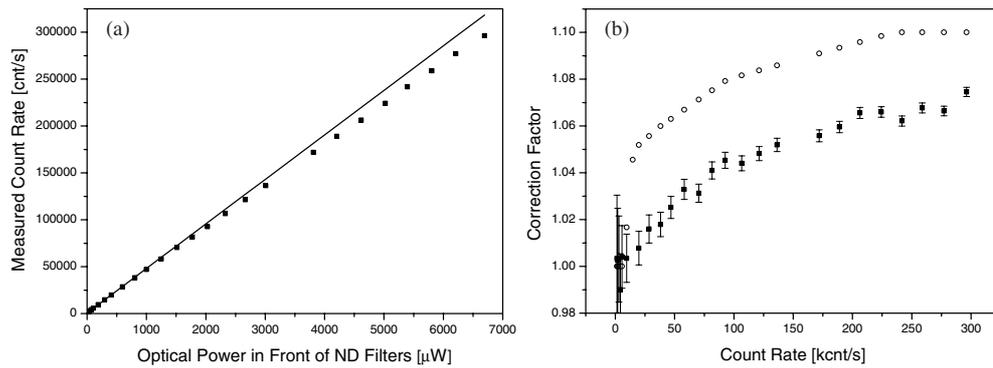
**Figure 2.** (a) Measured count rate for cw-light against optical power, i.e. transmission of the variable attenuation. The linear fit is included and for higher count rates a significant deviation of the measured data from a linear dependency is visible. The errors in the measured count rates are too small to be visible in the graph. (b) The correction factor calculated according to (6) against the measured count rate (■) in comparison to interpolated values from the data sheet (○).
