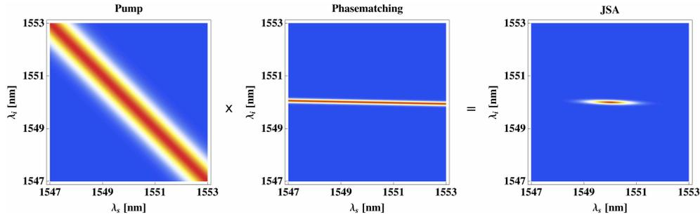
Fig. 2. Pump envelope, Phasematching function and JSA plotted in the Gaussian approximation without phase; Parameters: LN, type-I PDC, e-polarized rays, pump central wavelength  $\lambda_p = 775$  nm, FWHM of the pump intensity distribution  $\Delta\lambda_p = 0.58$  nm, waveguide dimensions:  $4 \mu\text{m} \times 4 \mu\text{m} \times 5$  mm, grating period  $\Lambda = 0.35 \mu\text{m}$ .
