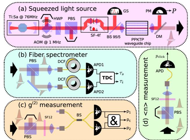
FIG. 1 (color online). Experimental setup: (a) PP-KTP waveguide source of two-mode squeezed vacuum states. (b) Fiber spectrometer for JSI measurement. (c)  $g^{(2)}$  measurement setup. (d) Mean photon number  $\langle n \rangle$  measurement.
