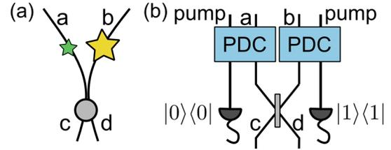
FIG. 4. Fundamental unit of the network (a) photon creation at a link  $b$  and no photon created at link  $a$ . (b) Experimental implementation using heralded parametric down-conversion.
