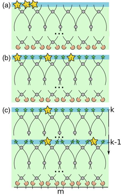
FIG. 1. Boson sampling networks for (a) boson sampling, (b) scattershot boson sampling, and (c) driven boson sampling with the state generation governed by a stack of  $k$  input layers each followed by an  $m \times m$  Haar-random unitary matrix  $\mathbf{U}_H^{(k)}$ . Green stars indicate all possible modes for injecting photons, yellow stars mark one possible ( $n = 3$ ) input state.
