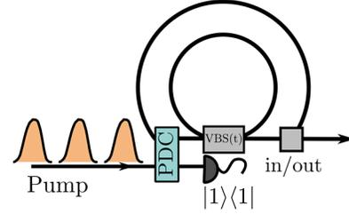
FIG. 6. Scheme of the time-multiplexing setup with a PDC source within the loop, adapting the scheme by Ref. [22]. The variable beam splitter  $VBS(t)$  implements all nodes in the network.
