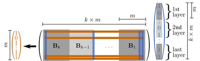
FIG. 3. Pictorial relationship of the input state to a particular measurement outcome  $|S_{\text{out}}\rangle$  due to matrix  $\mathbf{G}$  built from  $k$  blocks  $B_i$  of size  $m \times m$  [18].
