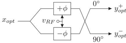
Fig. 3. Simplified architecture of the balanced MZM.
