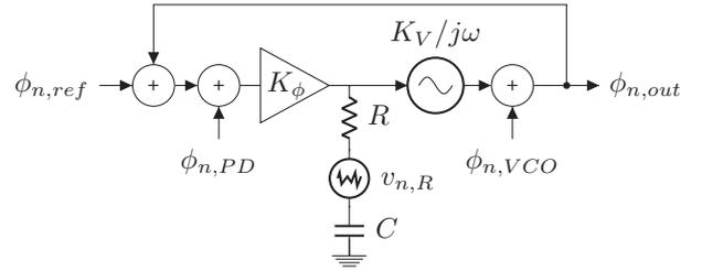
Fig. 5. Linear model of the OEPLL with the noise sources.
