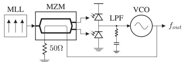
Fig. 1. Simplified block diagram of the Opto-Electronic PLL.
