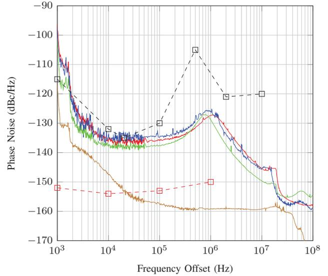
Fig. 7. Phase noise comparison: (brown) measured phase noise of 12<sup>th</sup> harmonic of the optical reference at 912 MHz, (red) measured phase noise of OEPLL at 10.032 GHz, (blue) measured phase noise at 7.6 GHz, (green) measured phase noise at 5.016 GHz, (dashed red) phase noise of [9] normalized to 10 GHz, (dashed black) phase noise of [11] at 10.17 GHz
