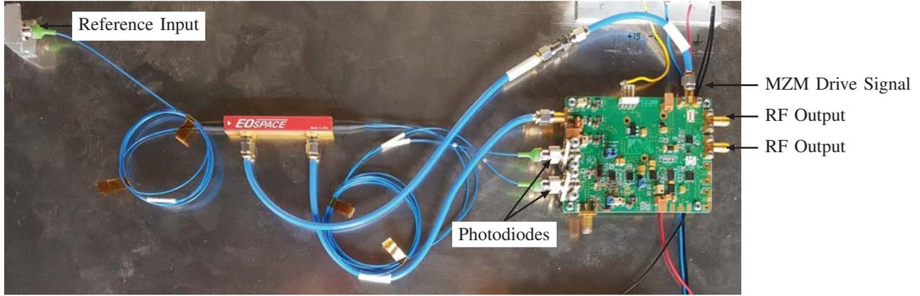
Fig. 6. Photograph of the developed unit.
