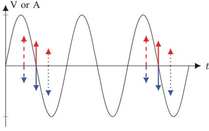
Fig. 2. (black) Excitation voltage of MZM, currents pulses generated at the upper (red) and lower (blue) photodiodes, when the reference and the VCO signals are in quadrature (solid), when reference has a phase lag (dashed) and when reference has a phase lead (dotted). This is a qualitative figure and the y-axis has units of Volts for the voltage waveform and Amperes for the current pulses.
