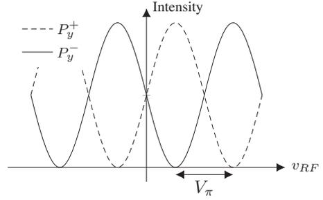
Fig. 4. The intensities of the outputs of the balanced MZM as a function of the excitation voltage.
