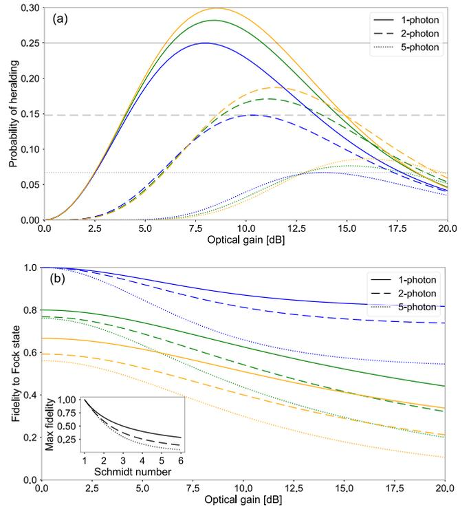
FIG. 3. (a) Heralding probability and (b) state fidelity vs the optical gain parameter. For these plots the heralding transmission value is kept constant at 0.9. Three different Schmidt values of 1, 1.5, and 2 are plotted (blue, green, and yellow curves, respectively). The inset (b) shows how the Schmidt number influences the maximal fidelity. Spectral modes up to  $K_{\max} = 35$  were considered for these calculations.
