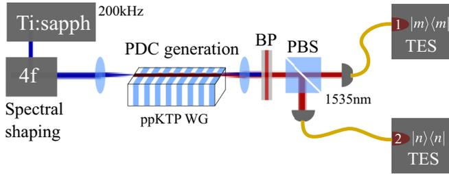
FIG. 4. Experimental setup as used in Ref. [16]. Pulsed light from a Ti:sapphire laser is spectrally filtered by a  $4f$  line and coupled into a periodically poled KTP waveguide. A bandpass (BP) filter is used to filter out the pump as well as to suppress sinc sidelobes of the phase-matching function. The signal and idler are split on a polarizing beam splitter (PBS) coupled into fibers and detected by intrinsic photon number resolving transition edge sensors (TESs).
