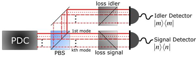
FIG. 1. Generating higher-order Fock states with type-II parametric down-conversion (PDC). The signal and idler mode are split one a polarizing beam splitter (PBS). Losses as well as spectral multimodeness are considered. For further information, see text.
