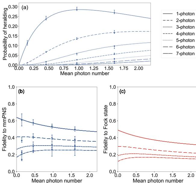
FIG. 5. Experimental data (points) for (a) the heralding probability and (b) the state fidelity without correcting for losses vs the measured mean photon number. Four different pump intensities were investigated. Colored lines show the theoretical values with  $K = 1.61$ ,  $\eta_i = 0.59$ , and  $\eta_s = 0.64$  as the only free parameters. In (b) the state fidelity to a mixed multimode photon number state is plotted whereas the calculated state fidelity to a Fock state is shown in (c).
