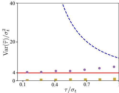
FIG. 4. Estimation errors for fully coherent signal ( $\gamma = 0$ ) per single total detection (purple circles, as in Fig. 3) and per single antisymmetric ( $\psi_a$ ) detection (brown squares). The quantum (red solid line) and classical incoherent (blue broken line) limits are also shown.
